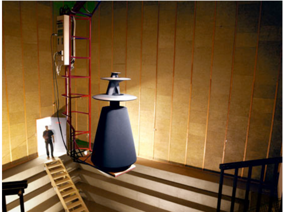
Bang & Olufsen's Cube, located at company headquarters in Denmark. The Cube is one of the world's largest, privately owned electroacoustic measurement facilities.
